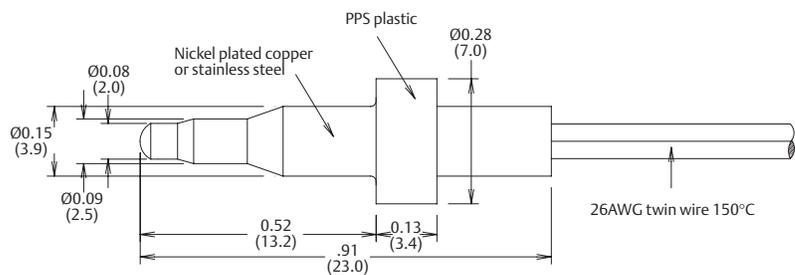
*Dimensions are shown in inches and (millimeters).*
