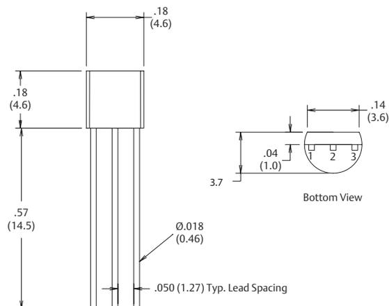
Dimensions are shown in inches and (millimeters).
