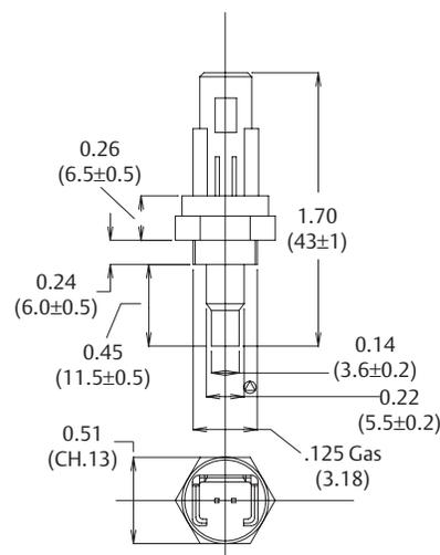
Dimensions are shown in inches and (millimeters).
