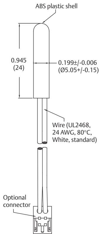
Dimensions are shown in inches and (millimeters).
