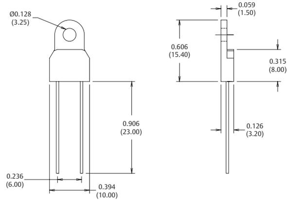
Dimensions are shown in inches and (millimeters).
