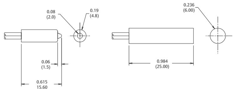
Dimensions are shown in inches and (millimeters)
