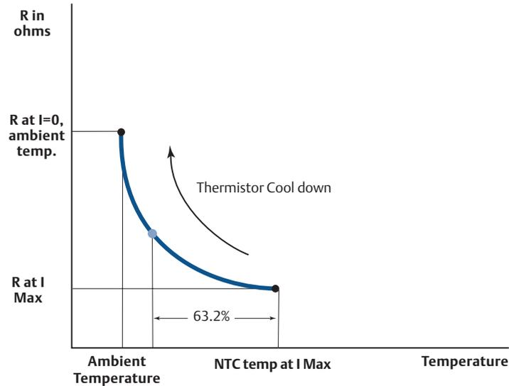
**Thermal Time Constant** – This is not how fast a thermistor will respond to a change in temperature. It is a method of comparing the relative speeds of thermistors with each other. By definition, the thermal time constant is the amount of time required for a thermistor to change 63.2% of the temperature difference between its initial and final sensing temperatures in a step-function change in temperature. This value is dependent on the sensing medium – still air, moving air, liquid, etc.
