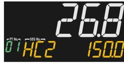
**Heater Break Alarm-2 Current Display (display only)**
