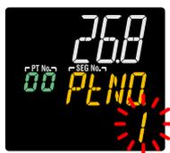
△▽ Press the Up/Down arrow keys to display the required setpoint.
