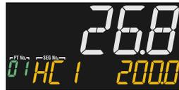
**Heater Break Alarm-1 Current Display (display only)**
