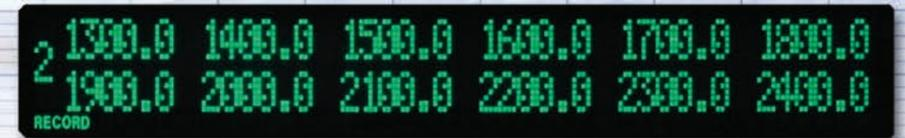
Two groups are alternately displayed: 18 dot model 1Gr (1 to 12ch), 2Gr (13 to 18ch)
