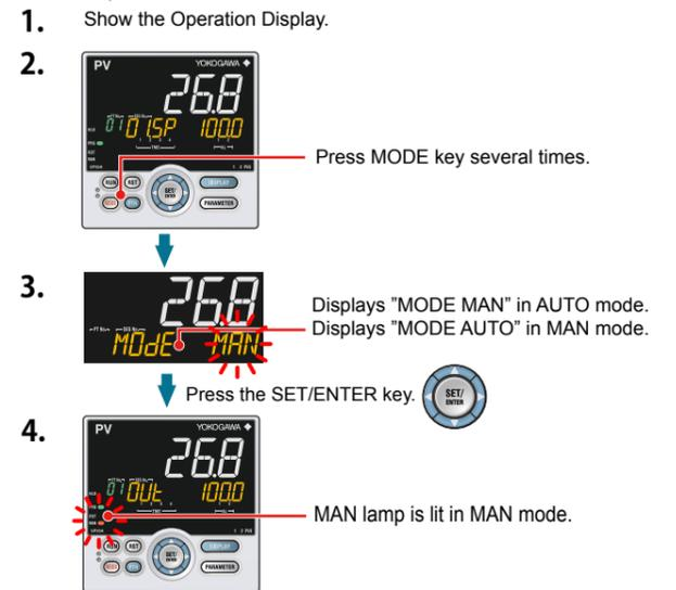
When AUTO is switched into MAN, the control output value in AUTO mode is held. The controller can be operated manually from the hold value. If the manual preset output is set (MPON parameter ≠ OFF), the controller can be operated manually from the arbitrary output value (MPO1 to MPO5 parameters).
