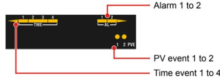
**Operation Display Switching Diagram**
