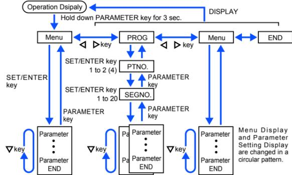
The parameter groups can be switched using ◀ ▶ keys. Move to the Setup Parameter Setting Display: Hold down the PARAMETER key and the Left arrow key simultaneously for 3 sec.
