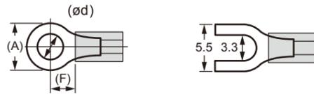
Recommended tightening torque: 0.6 N·m
