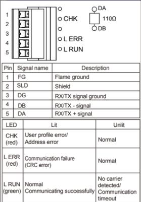
If the UT is located at the end of a segment for the CC-Link communication wiring, terminating resistors are separately needed. These are to be prepared by users. (110 Ω: 1 pc.)
