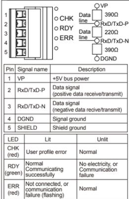
If the UT is located at the end of a segment for the PROFIBUS communication wiring, terminating resistors are separately needed. These are to be prepared by users. (390 Ω: 2 pcs. 220 Ω: 1 pc., or an active terminator.)
