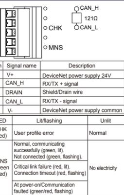
If the UT is located at the end of a segment for the DeviceNet communication wiring, terminating resistors are separately needed. These are to be prepared by users. (121 Ω: 1 pc.)
