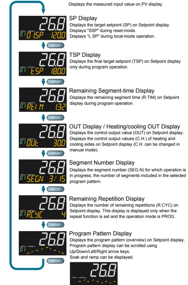
After showing the Program Pattern Display, press the DISPLAY key to show the following displays conditionally. For details, see User's Manual.
