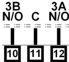
Figure 33. Plug-in Module Slot 3 - Dual Relay Module
