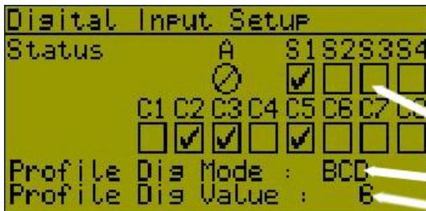
A diagnostic screen assists commissioning and fault finding by showing the current signal state for all digital inputs.
