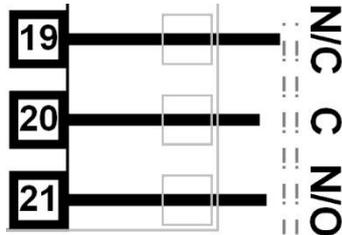
Figure 22. Plug-in Module Slot 1 – Single Relay Module
