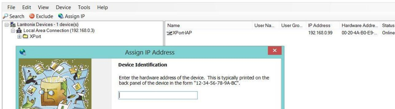
The existing IP and Hardware (MAC) addresses are shown for the instruments found.
