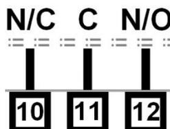
Figure 32. Plug-in Module Slot 3 – Single Relay Module
