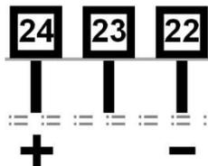
Figure 31. Plug-in Module Slot 2 - Transmitter Power Supply Module
