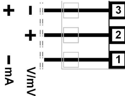
Figure 13. Input 1 - DC Volt, mV & mA Connections
