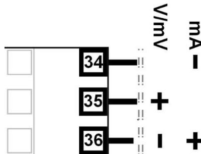
Figure 16. Input 2 - DC Volt, mV & mA Connections
