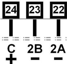
Figure 29. Plug-in Module Slot 2 – Dual SSR Driver Module
