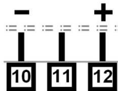
Figure 34. Plug-in Module Slot 3 – Single SSR Driver Module
