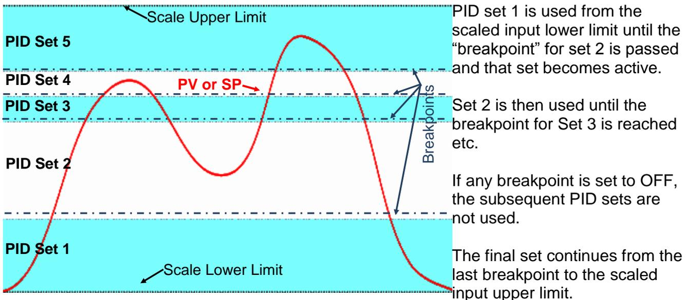
Gain Scheduling breakpoints can be selected to switch PID sets with a change in the current setpoint value, or the current process value.
