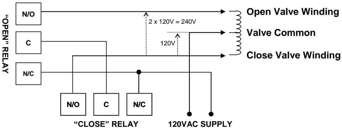
Figure 42. Interlocking of Valve Motor Drive Relays
