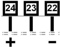
Figure 28. Plug-in Module Slot 2 – Single SSR Driver Module
