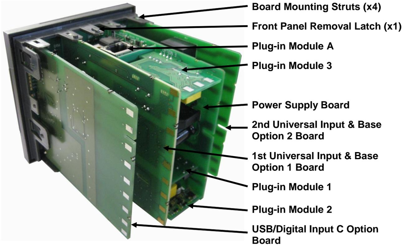
Figure 3. Rear view (uncased) & board positions
