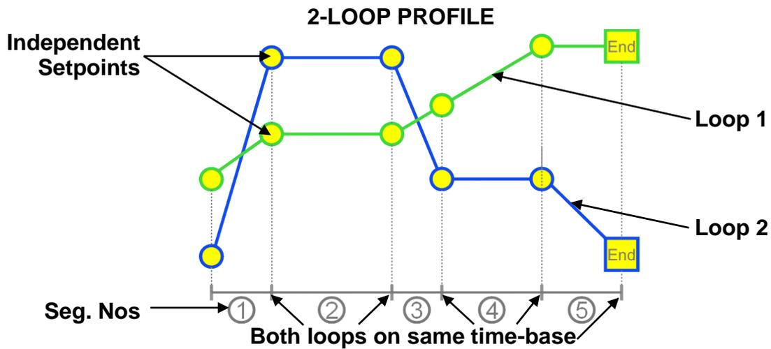
Seg. ① & ② shows a ramp and a dwell with the shared time base. The ramp direction can be different (Seg. ③), and although one loop cannot ramp while the other dwells, a "dwell" is achieved by a ramp with its final setpoint value at the same value as the previous segment (Seg. ④). Similarly, if only one loop is to Step to a new value, make the other "step" to its existing setpoint value. If you later change the previous setpoint, you may have to change both segments.
