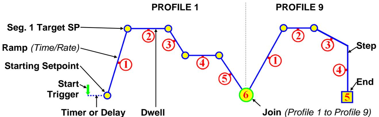
Figure 49. Profile Starting and Standard Segment Types
