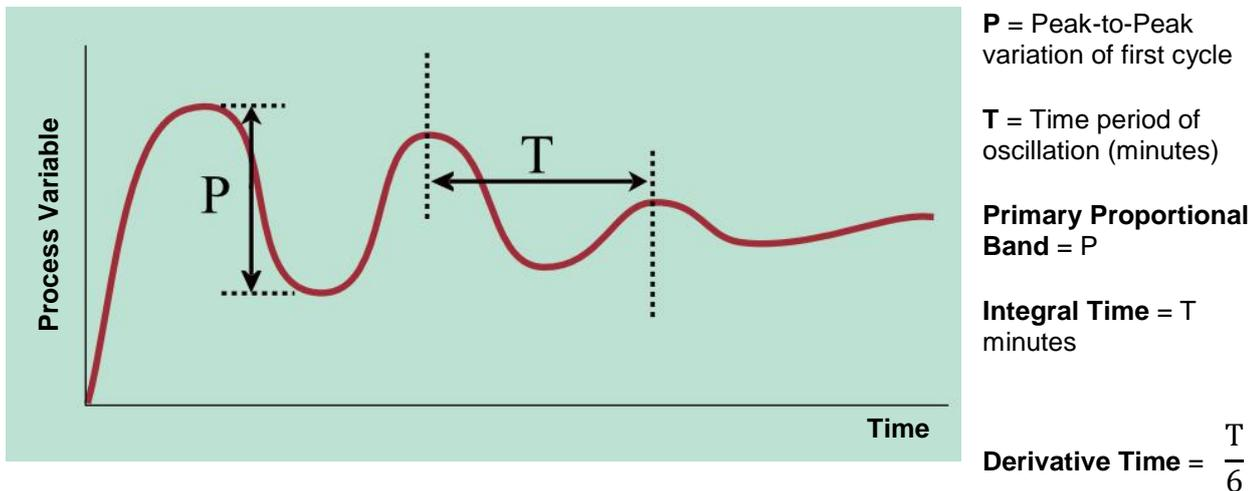
Figure 60. Manually Tuning - PID with Primary Output
