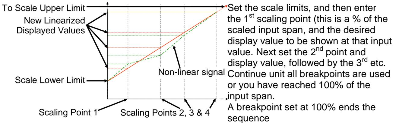
Figure 46. Multi-point Scaling
