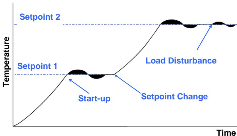
Figure 59. Self-Tune Operation
