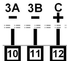
**Plug-in Module Slot 3 - Triac Output Module**
