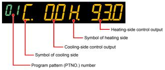
Up arrow key: concurrently decreases cooling-side control output and increases heating-side control output.
