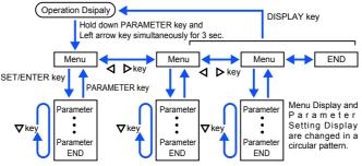
Move to the Operation Parameter Setting Display: Hold down the PARAMETER key for 3 sec.
