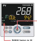
Up arrow key: increases control output Down arrow key: decreases control output
