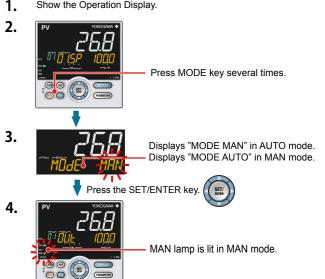
When AUTO is switched into MAN, the control output value in AUTO mode is held. The controller can be operated manually from the hold value.
