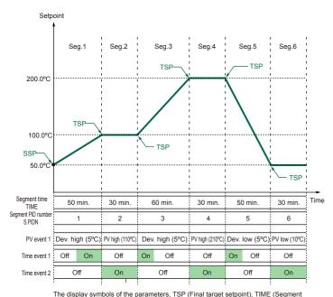
The display symbols of the parameters, TSP (Final target setpoint), TIME (Segment time setting), and S.PID (Segmet PID number selection) are the same in each segment. However, the segment can be recognized by the number displayed on the Symbol display.
