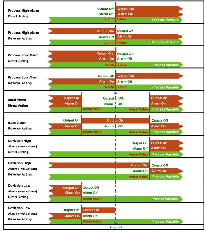
Figure 64. Alarm Operation
