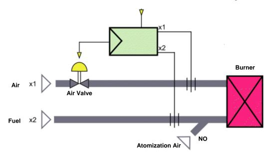
Figure 48. Ratio Control Example
