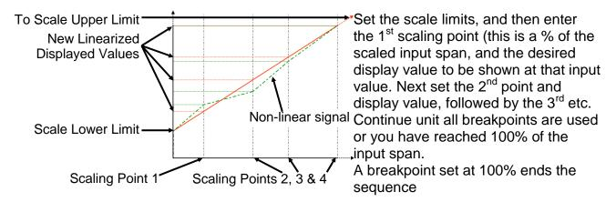
Figure 46. Multi-point Scaling
