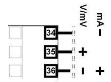
Figure 16. Input 2 - DC Volt, mV & mA Connections
