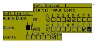
The four soft digital inputs can be configured by combining physical inputs, alarms & events using Boolean logic. Input AND selections are then globally OR'd with the input OR selections, the alarms & the events. By using the invert inputs function, NAND & NOR equivalents can be created.
