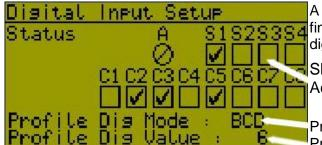
A diagnostic screen assists commissioning and fault finding by showing the current signal state for all digital inputs.
