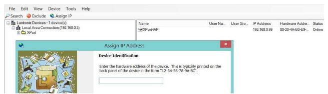
The existing IP and Hardware (MAC) addresses are shown for the instruments found.
