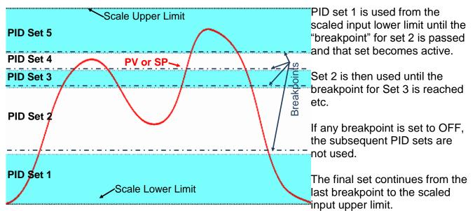
Gain Scheduling breakpoints can be selected to switch PID sets with a change in the current setpoint value, or the current process value.
