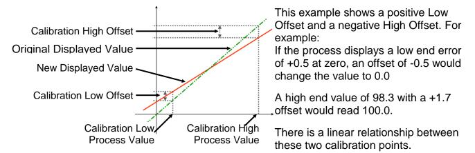
Figure 45. Two Point Calibration
