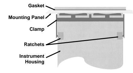
1. Insert instrument into the panel cut-out.
