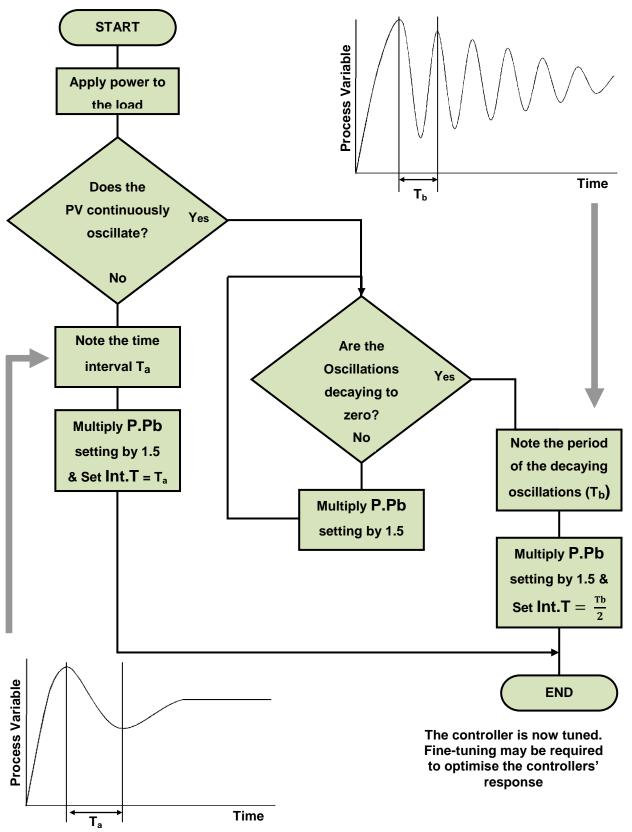
This method can also be used to tune PID loops. Set Derivative to approx. Ta / 4
