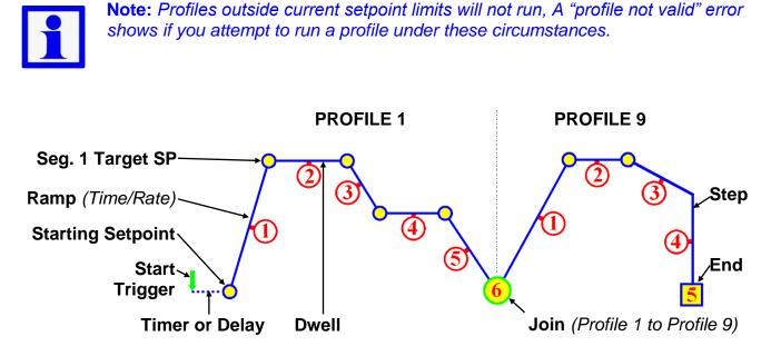
Figure 49. Profile Starting and Standard Segment Types
