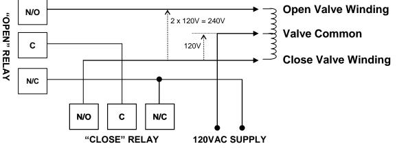
Figure 42. Interlocking of Valve Motor Drive Relays
