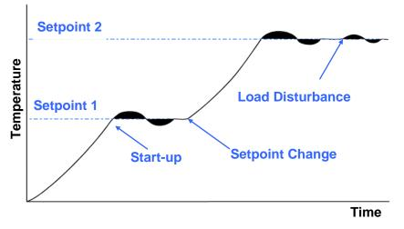
Figure 59. Self-Tune Operation
