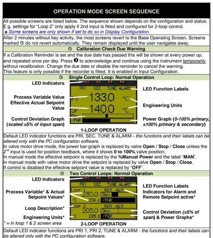
In valve motor drive mode, the power bar-graph is replaced by valve **Open / Stop / Close**. In manual mode the effective setpoints are replaced by the **%Manual Power** and the label **"MAN**". In manual mode with valve motor drive the setpoint is replaced by valve **Open / Stop / Close**. If control is disabled the effective setpoint value of that loop is replaced by "**OFF**".
