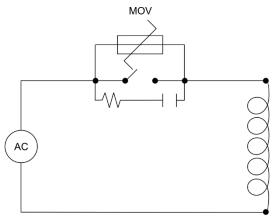
Figure 6. Contact noise suppression
