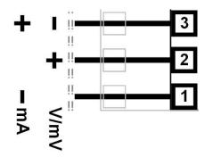
Figure 13. Input 1 - DC Volt, mV & mA Connections
