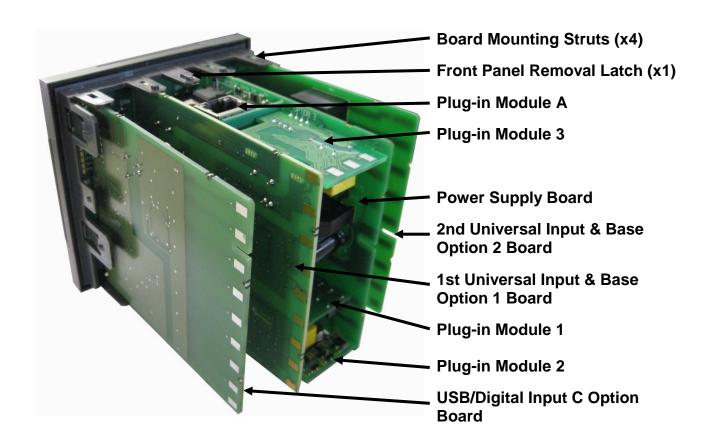
Figure 3. Rear view (uncased) & board positions
