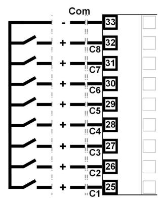
Figure 41. Option C - Multiple Digital Inputs C1 to C8
